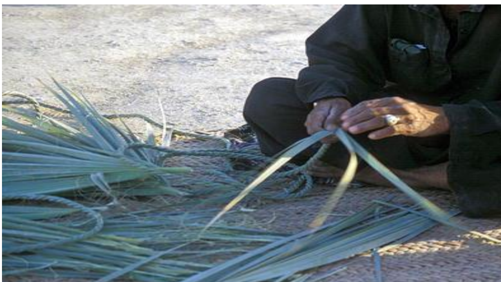
Rope-making by plying (or twisting) four leaf strands of Nannorhops Ritchieana The Rope-maker sits on a mat equally produced from palm leaves somewhere in Makran
