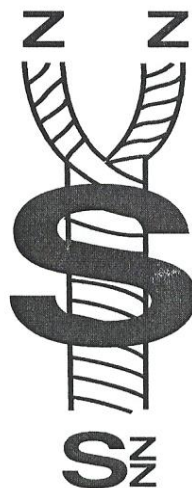
Structure of a double standard S-lay cord obtained by the association of two Z-lay yarns (Courtesy Archaeol Anthropol Sci 2012)
